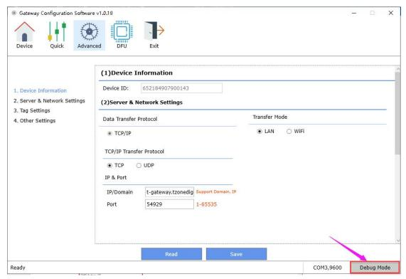
2) In debug mode, the Gateway parameters are configured directly by commands. Note: After writing the commands, please click "send". After sending (Please refer to the command list for more detailed).
